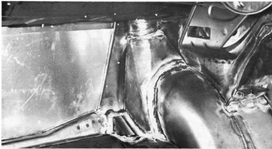
Works turret viewed from inside boot. Damper top nut access is from inside cockpit.
